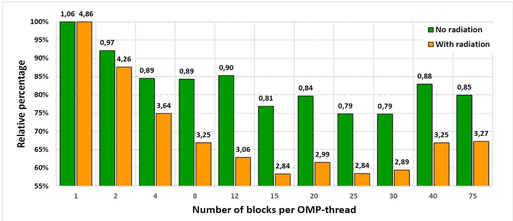
Cray XC40. The numbers above the bars show the wall-clock time in seconds.
